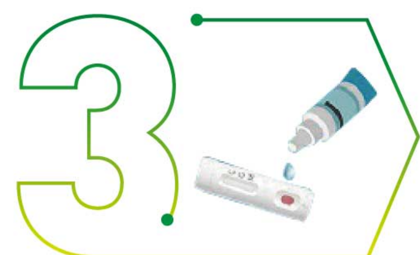
Place 2-3 drops of buffer in sample well
